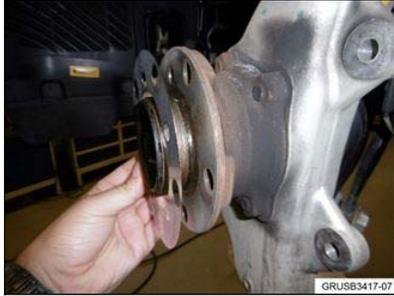
5. Install “friction ring” on wheel bearing flange as shown.
