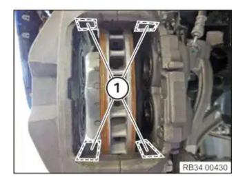
To prevent damage to the surface coating, do not clean the guide surfaces (1) for the brake pads on the brake calliper mechanically, if possible.
