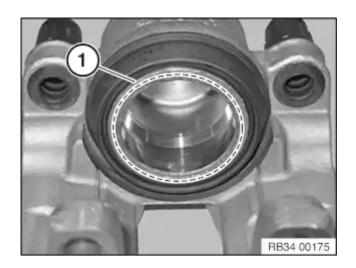
Clean contact surface (1) of brake piston with brake cleaner and apply a thin coating of brake pad paste.
