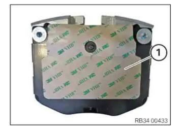
Remove the protective film of the adhesive layer (1) from the brake pads.
