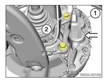
Install the brake caliper (1) in direction of arrow.
