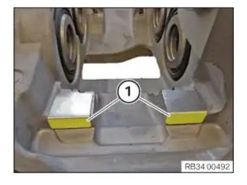
So as not to damage the surface coating, if possible do not mechanically clean the guide surfaces for the brake pads on the brake caliper mounting bracket.
