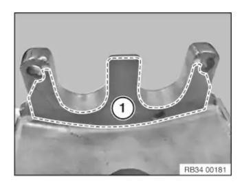
Clean contact surface (1) and brake caliper with brake cleaner and apply a thin coating of brake pad paste.
