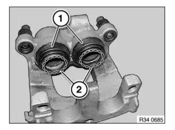
Clean contact surface (2) of brake piston with brake cleaner and apply a thin coating of brake pad paste.
