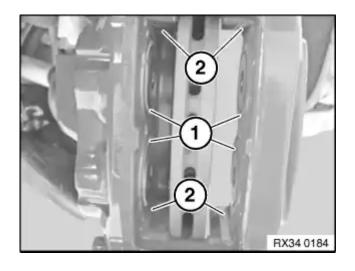
Check dust boot (1) for damage and replace if necessary. Clean brake caliper compartments (2) and apply a thin coating of brake pad paste.
