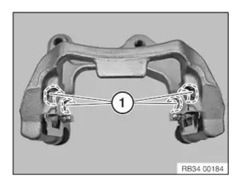
So as not to damage the surface coating, <u>if possible do not mechanically clean</u> the guide surface (1) for the brake pads on the brake caliper mounting bracket. Clean guide surface (1) with brake cleaner and apply a thin coating of brake pad paste.
