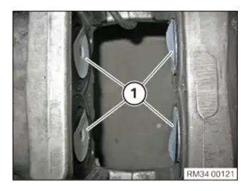
Insert the claw plates (1) into the brake pistons.
