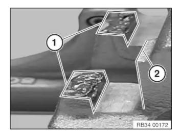
So as not to damage the surface coating, <u>if possible do not mechanically clean</u> the guide surfaces (1) for the brake pads on the brake caliper mounting bracket. Clean guide surfaces (1) with brake cleaner and apply a thin coating of brake pad paste.
