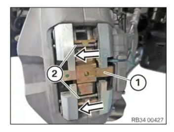
Insert brake pads in the brake caliper, making sure the adhesive layer does not touch the brake pistons.
