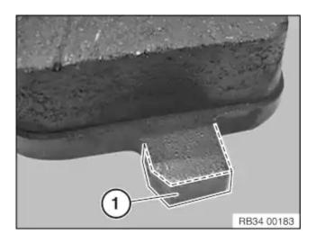
Apply a thin coating of brake pad paste to both sides of T-head of brake pad in area (1).
