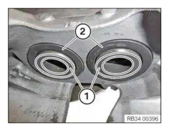
Clean the contact surface (1) of the brake piston (4 pieces) with brake cleaner.
