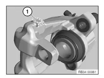
Clean contact surfaces (1) of T-heads/brake calliper housing with brake cleaner and apply a thin coating of brake pad paste.
