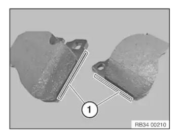
Lightly coat the brake pad contact surface on both sides in area (1) with brake pad paste.
