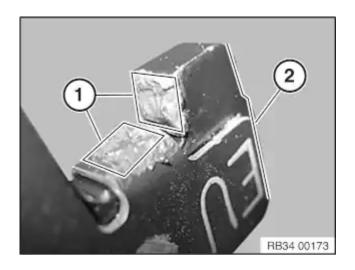
Apply a thin coating of brake pad paste to T-head of inner brake pad in area (1) and (2).
