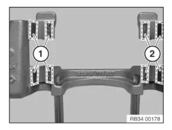
So as not to damage the surface coating, <u>if possible do not mechanically clean</u> the guide surfaces (1 and 2) for the brake pads on the brake calliper mounting bracket. Clean guide surfaces (1 and 2) with brake cleaner and apply a thin coating of brake pad paste.
