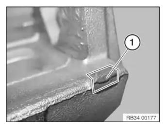
Clean contact surfaces (1) of T-heads/brake calliper housing with brake cleaner and apply a thin coating of brake pad paste.
