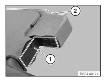
Apply a thin coating of brake pad paste to T-head of outer brake pad in area (1) and (2).
