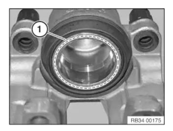
Clean contact surface (1) of brake piston with brake cleaner and apply a thin coating of brake pad paste.
