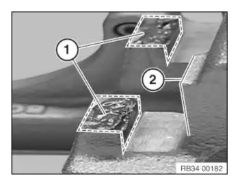
So as not to damage the surface coating, <u>if possible do not mechanically clean</u> the guide surfaces (1 and 2) for the brake pads on the brake calliper mounting bracket. Clean guide surfaces (1 and 2) with brake cleaner and apply a thin coating of brake pad paste.
