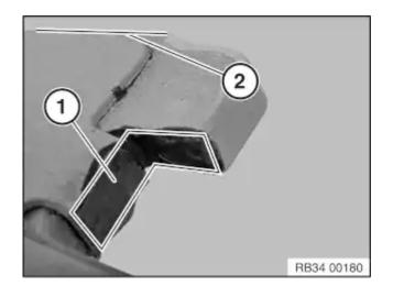
Lightly coat the T-head of the outer brake pad with brake pad paste in area (1 and 2).
