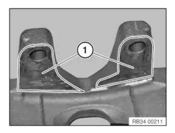
Clean contact surface (1) of brake caliper with brake cleaner and apply a thin coating of brake pad paste.
