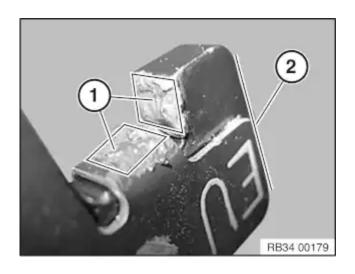
Lightly coat the T-head of the inner brake pad with brake pad paste in area (1 and 2).
