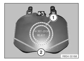
Lightly coat both sides of the contact surface in area (1 and 2) with brake pad paste.
