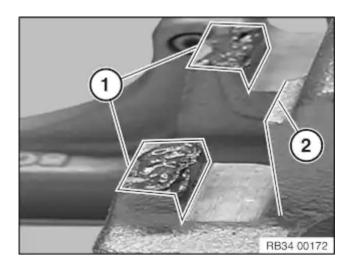
So as not to damage the surface coating, <u>if possible do not mechanically clean</u> the guide surfaces (1) for the brake pads on the brake caliper mounting bracket. Clean guide surfaces (1 and 2) with brake cleaner and apply a thin coating of brake pad paste.
