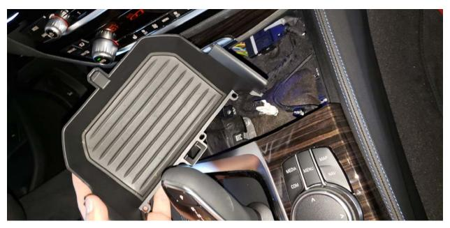
8. Remove 2 T20 screws from passenger side trim making space to fish the wire for new tray.
