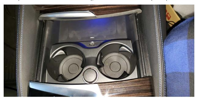
15. Connect the supplied extra cable to the charging tray connection on the passenger side.
