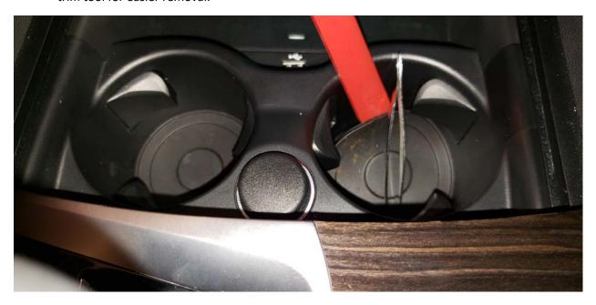
2. Remove both T20 screws from cup holders.
