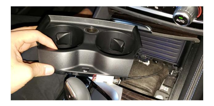
13. Side back the cup holder into place, this will also lock the charging tray in position so those charging tray screws won't matter.
