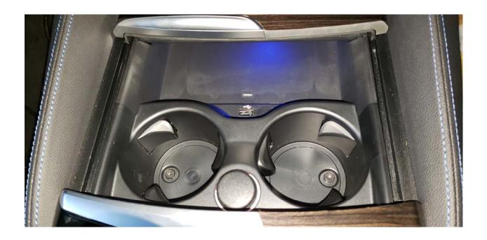
3. Side Trim tool in the gaps and push down on each clip and fliting it from the front to remove the cup holder.
