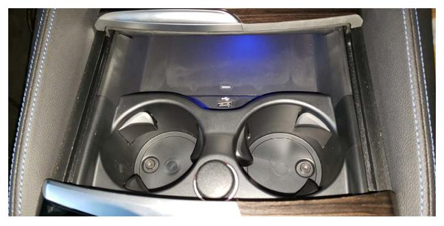
14. Screw back the 2 T20 screws in the cup holder and drop back the rubber inserts. (If your usb port looks crooked like mine don't worry, Just insert a usb stick to fix the position)
