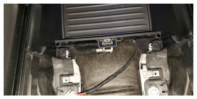
6. Carefully unclip usb port from regular tray making sure not to damage it.
