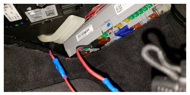
18. Connect the fuse tap to F59 or F51 Empty Fuse on the passenger Side Fuse box. ( You can also connect to a same fuse tap if you have a radar or dash cam)
