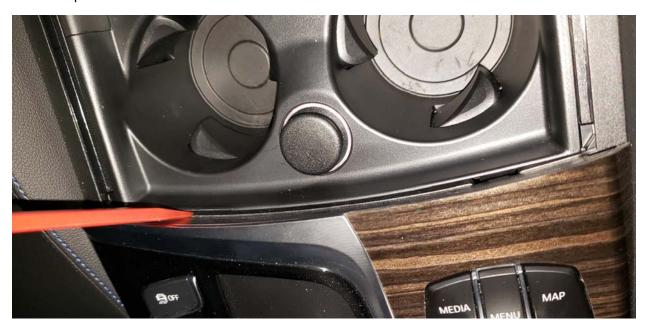
4. Remove wire clip connecting from cup holder for cigarette lighter connection and set aside.
