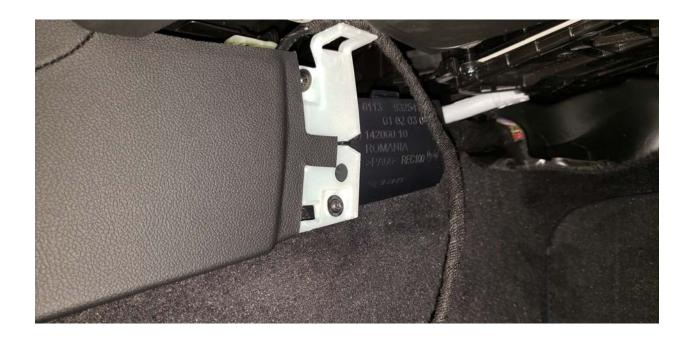
9. Tape the end clip on the new charging tray connection to a piece for trim tool or something so you can fish the wire out on the passenger side without damaging the charging tray connection.
