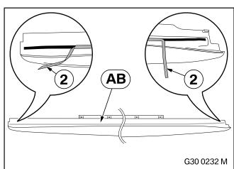
Release a little of the adhesive backing film (2) on both sides of the "Matt black side sill add-on section, left" **AB**.
