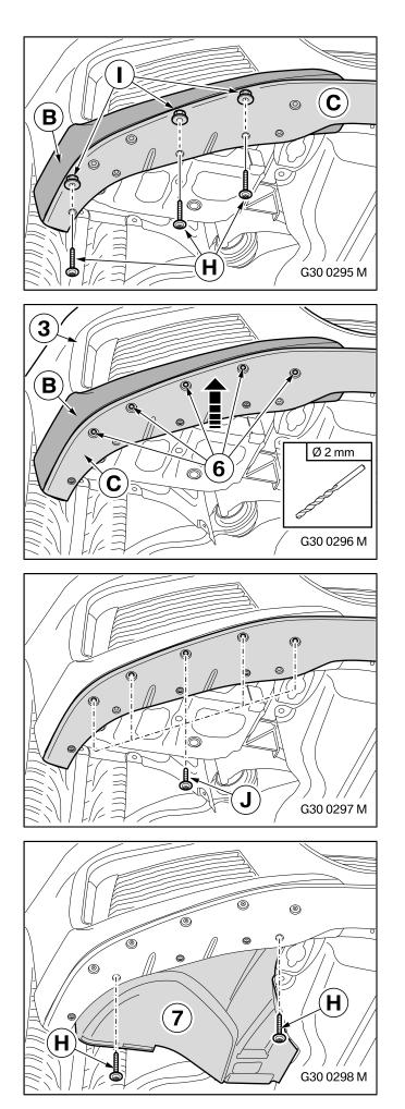
Align the "Carbon front add-on section" **C** and install it with screws **H** and plastic cap nuts with washer **I**. Ensure that the gaps to the "Carbon front add-on section, left" **A** and "Carbon front add-on section, right" **B** are uniform.
