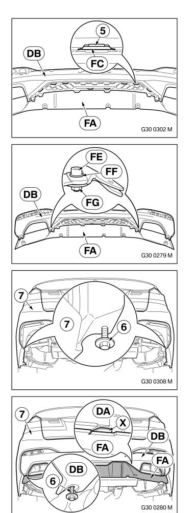
Insert the "Carbon rear diffuser" **FA** with lugs (5) into the "Matt black rear bumper trim" **DB**.
