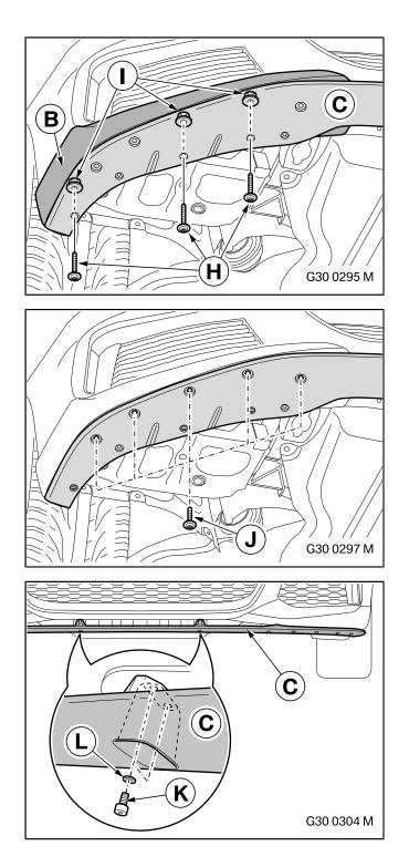
Install the "Carbon front add-on section" **C** with screws **H** and plastic cap nuts with washer **I**.
