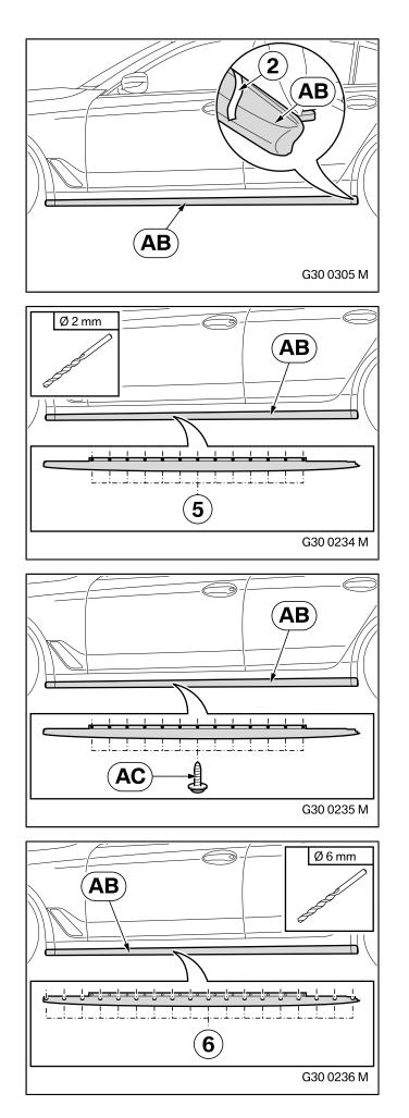
Carefully remove the adhesive backing film (2) from the outside inwards and firmly press on the "Matt black side sill add-on section, left" AB.
