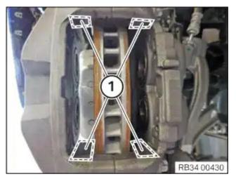
Clean the contact surfaces (1) for the brake pads on the brake caliper with brake cleaner.
