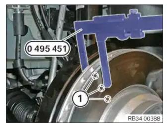
• Check minimum brake disc thickness:
