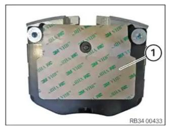
Remove the protective film of the adhesive layer(1) at the brake pads.
