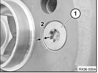
Check that the mounting bolt (1) for the brake disc is securely seated.
