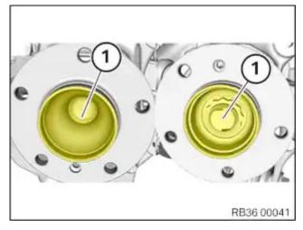
Lightly grease the front and rear wheel hubs in this area (1) to protect from corrosion.
