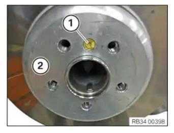
Clean contact surface of wheel hub thoroughly and remove any traces of rust if necessary.
