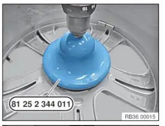
Remove dirt, grease residues and corrosion from the contact surface with a drill and the special tool 2 344 011.
