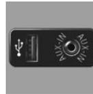
Connect the headphones or line-out connector of the mobile audio device to the AUX-IN port.
