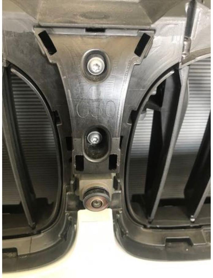
Step 3: Install the painted cover in reverse and install the kidney grill back in place.
