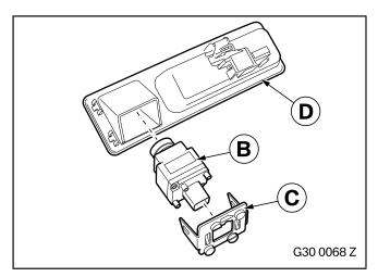
Install rear view camera  ${\bf B}$  with bracket  ${\bf C}$  in the tailgate button  ${\bf D}$ .
