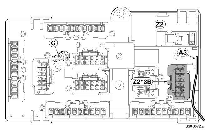
Connect branch **A3**, RT/VI cable, using miniature connector **G** to the GN cable from PIN 11 on plug **Z2\*3B** on rear right fuse box**Z2**.
