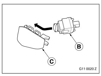
Clip the rear view camera **B** into holder **C**.
