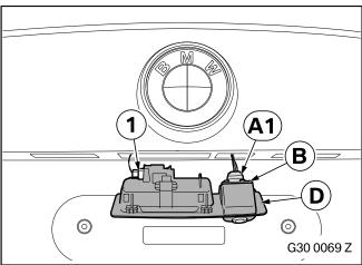
Connect branch **A1**, SW 8-pin socket housing, to rear view camera **B**.
