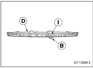
Secure the rear view camera  ${\bf B}$  using a fillister head screw  ${\bf I}$  to the handle strip  ${\bf D}$ .
