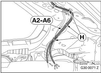
Route branches **A2-A6** along the D pillar to righthand side of the luggage compartment and secure them to the standard wiring harness using cable ties **H**.
