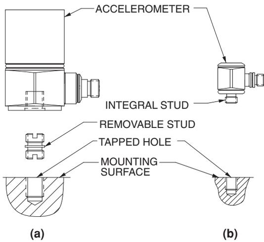
Figure 3: The threaded stud mount
