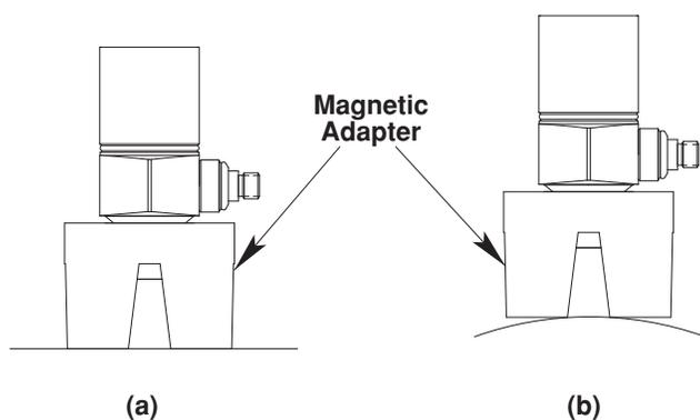
Figure 6: Magnetic mounting adapters
