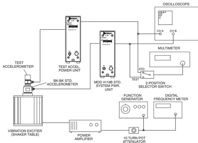
Figure 1: Back-to-back calibration set-up
