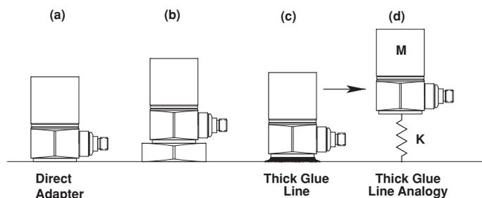
Figure 5: The adhesive mount, direct and with adapter
