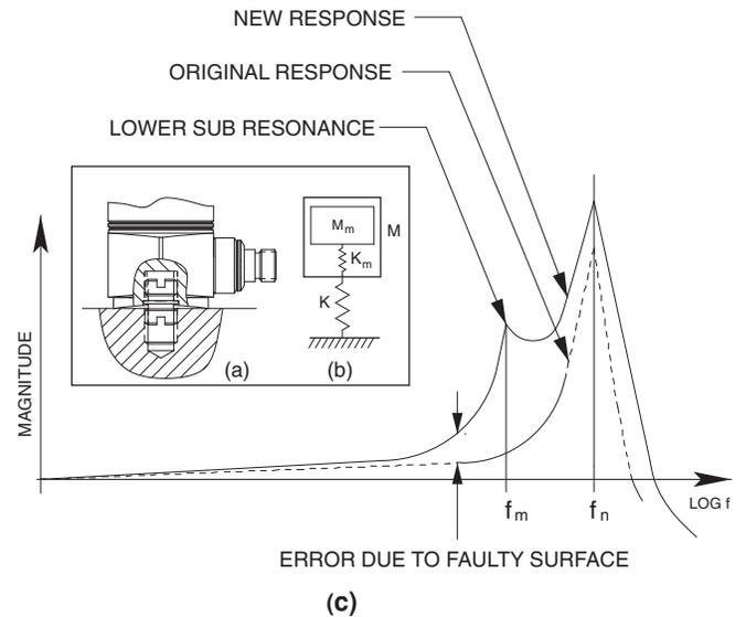
Figure 4: Non-flat accelerometer mounting surface
