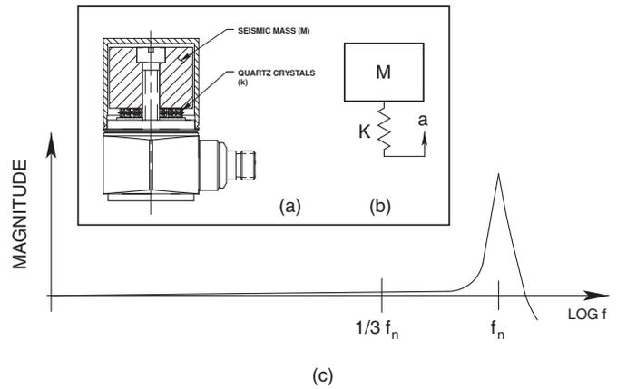
Figure 2: The accelerometer as a spring-mass system.
