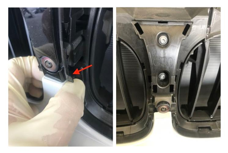
Step 3: Install the painted cover in reverse and install the kidney grill back in place.
