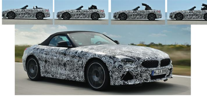
roof up or down. Additionally, the roof can be raised or lowered in ten seconds at speeds up to 30 mph.
